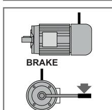
Reducers are not to be considered fail safe or self-locking devices. If these features are required, a properly sized, independent holding device should be used. Reducers should not be used as a brake. Any brakes that are used in conjunction with a reducer must be sized or positioned in such a way so as to not subject the reducer to loads beyond the catalog rating.
