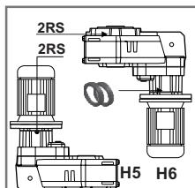
Please specify when ordering if reducer are used in Vertical H5 or H6 mounting position. We normally mount a 2RS self lubricated bearings ( see picture ) for V6 mounting we recommend double oil seals in the input side H6 positions is not recommended for 2 poles motors
