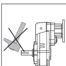
When mounting pinions, pulleys or couplings on the reducer's shaft, protect the bearings from impact by using the appropriate pullers and threaded holes in the end of the reducer shaft.
