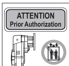
It's compulsory to request HYDRO-MEC authorization to use our COMPACT-GEAR when the units are used in a man lift or people moving devices.
