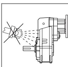
If the reducer is to be painted, protect machined surfaces and oil seals from over-spray.
