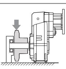
For very heavy radial load, additional output shaft support may be required to prevent premature bearing failure or shaft breakage from bending fatigue.
