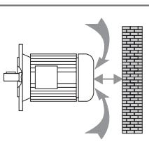
Make sure there is sufficient space between any obstructions and the motor's air intake area to provide adequate cooling for the motor.
