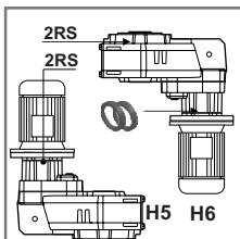
Do not change mounting positions without contacting our factory. Altering the mounting position may require special lubrication provisions which must be installed from the factory. When reducers are mounted in positions H5 or H6 and used in continuous duty applications, replace the upper bearing with a self-lubricating style bearing, and we suggest double input seal for H6.
