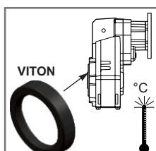
In case of high temperatures we suggest to use FPM (fkm) Oil seals in the output shaft.
