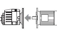
When mounting a motor to reducers, the fastening bolts should not be tightened until both the reducer flange and motor face are in contact. When mounting is complete check by manually rotating the fan to be sure the assembly turns freely.
