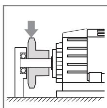
For very heavy radial load, additional output shaft support may be required to prevent premature bearing failure or shaft breakage from bending fatigue.
