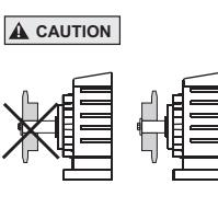
Make sure that mounting of pulleys or pinions does not create over hung loads exceeding the capacity of the reducer.
