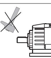
When mounting pinions, pulleys or couplings on the reducer's shaft, protect the bearings from impact by using the appropriate pullers and threaded holes in the end of the reducer shaft.
