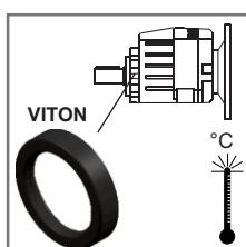
In case of high temperatures we suggest to use FPM (fkm) Oil seals in the output shaft.
