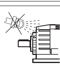
If the reducer is to be painted, protect machined surfaces and oil seals from over-spray.
