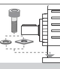
Mount the reducer on a flat surface free of vibration. If high overhung loads are expected, it is advisable to reinforce bolt heads with washers as shown in picture.
