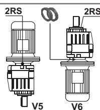
Do not change mounting positions without contacting our factory. Altering the mounting position may require special lubrication provisions which must be installed from the factory. When reducers are mounted in positions V5 or V6 and used in continuous duty applications, replace the upper bearing with a self lubricated style bearing, and we suggest double input seal for V6.
