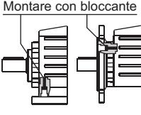
In applications where multiple starts, stops or reverses occurs, it is recommended to block the fastening bolts of the output flange and feet.
